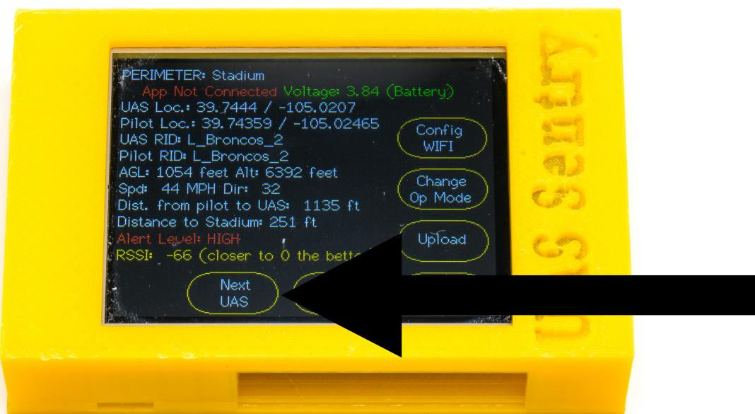
Most drones use channel 6 for transmitting Wifi RID packets. However, the standard does not specify that channel 6 must be used so the Sentry also monitors the other channels.
