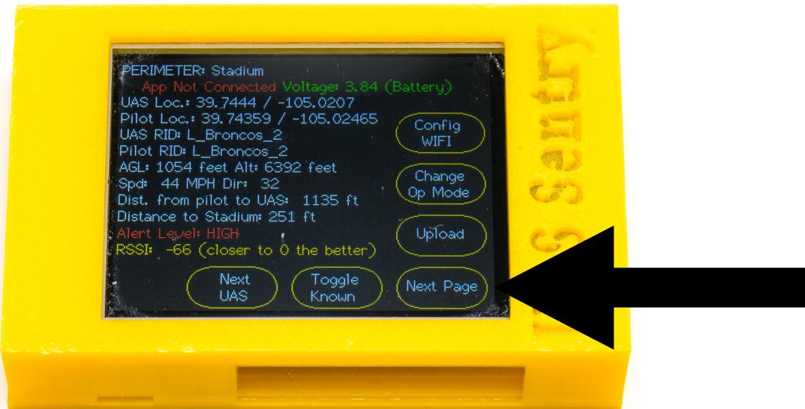
If more than 1 drone is detected you can tap the Next UAS button to see data about the next drone. When a particular drone is no longer being detected the color of the data being displayed will be orange.
