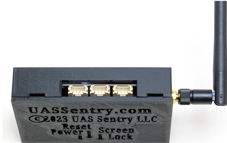
On the top of the unit are three connectors which are reserved for future use (e.g., LEDs, Alarms, etc.).
